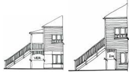
Figure 6.70 — Appropriate enclosures to the ground floor
