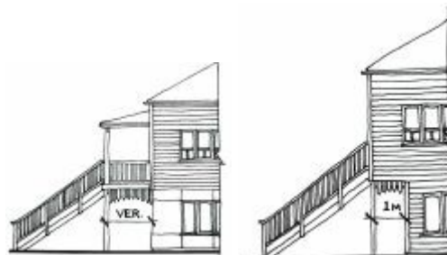
Figure 6.74 - Appropriate enclosures to the ground floor
