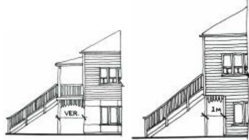
Figure 6.80 — Appropriate enclosures to the ground floor
